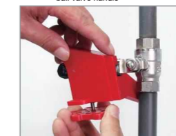
Step 2: Tighten the clamp to grip the ball valve handle
